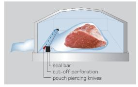
High Pressure Double Biactive Sealing and Spring Loaded Resistance Wires are standard. Tough and reliable seals despite wrinkles, moisture and grease in the seal area. Springs keep the resistance wires taut during continuous production, increasing the working life of resistance wires and teflon.
