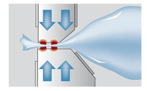
The double biactive high-pressure sealing as well as spring-loaded resistance wires are an integral part of the standard equipment and guarantee safe and reliable seals.
